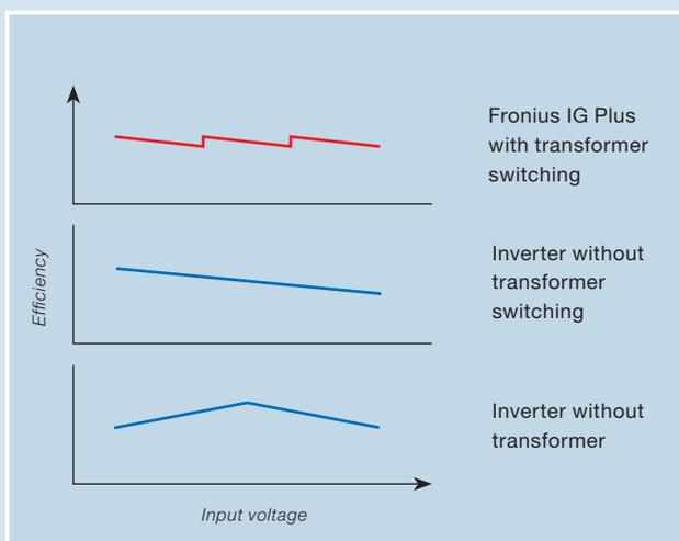
**MIX™ concept.** You will get the maximum power harvest out of partial load ranges, e.g. on cloudy days, through a clever combination of multiple power stages in each inverter. The power stages in the Fronius inverters divide up the work depending on the operating hours.
